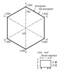
Test Item: G5NB-1A4-EL-HA 24 VDC Number of Relays: 5 pcs Test Method: Shock was applied 3 times in 6 directions along 3 axes and the level at which shock caused malfunction was measured.
