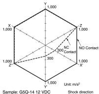
Number of Relays: 5 pcs Test conditions: Shock is applied in  $\pm X$ ,  $\pm Y$ , and  $\pm Z$  directions three times each with without energizing the Relays to check the number of malfunctions. Requirement: None malfuction 100 m/s<sup>2</sup>
