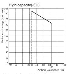
Note. The Maximum coil voltage refers to the maximum value in a varying range of operating power voltage, not a continuous voltage.
