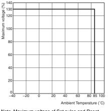
Note. Maximum voltage of Set pulse and Reset pulse at duty factor 10%.
