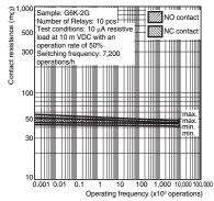
The test was conducted at an ambient temperature of 23°C. \*1. \*2. The contact resistance data are periodically measured reference values and are not values from each monitoring operation. Contact resistance values will vary
