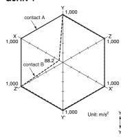
Sample: G6RN-1 24 VDC Number of Relays: 5 pcs Test conditions: The value at which malfunction occurred was measured after applying shock to the test piece 3 times each in 6 directions along 3 axes. Standard value: 100m/s² at contact A,
