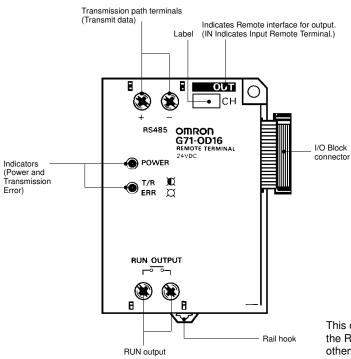
This output turns ON when the programmable controller is in the RUN or MONITOR mode and no error has occurred; otherwise OFF.
