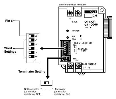
Note: The terminator setting also sets the termination resistance. Be sure to set only one terminator per Remote I/O Master Unit and be sure it is the Unit farthest from the Master. (Set to OFF at the factory).
