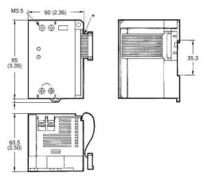
\*A flat cable with a length of 85 mm can be used.
