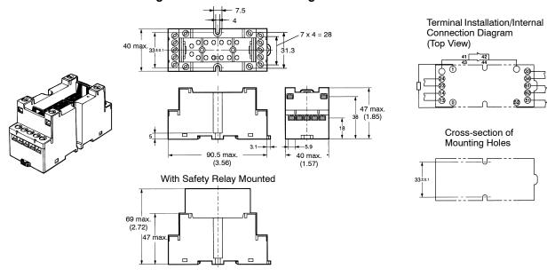
P7S-14A Panel-mounting Socket (Solder Terminals)
