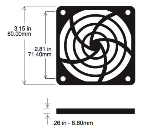
Material Plastic - reinforced ABS UL approved Rating UL94V-O
