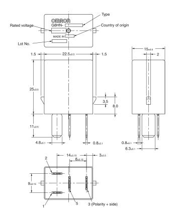
Terminal arrangement / Internal connections (BOTTOM VIEW)
