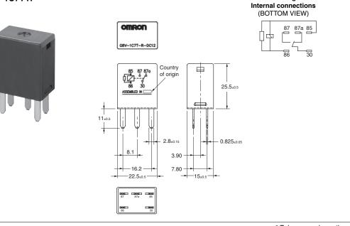
\* Tolerance unless otherwise specified Less than 1 mm: ±0.1 mm Less than 1 to 3 mm: ±0.2 mm 3 mm or more: ±0.3 mm
