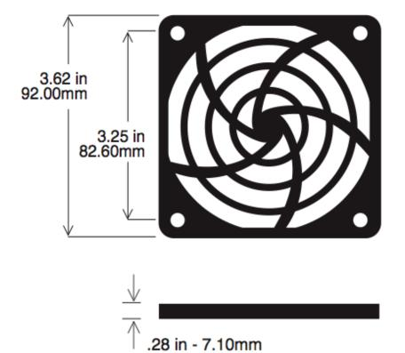
Material Plastic - reinforced ABS UL approved Rating UL94V-O
