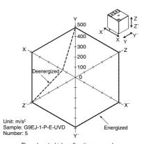
The value at which malfunction occurred was measured after applying shock to the test piece 3 times each in 6 directions along 3 axes.
