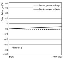
Characteristics were measured after applying a shock of 490 m/s $^{2}$  to the test piece 3 times each in 6 directions along 3 axes.
