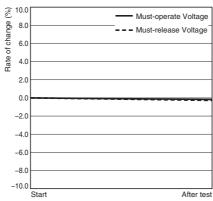
Characteristics were measured after applying vibration at a frequency of 5 to 200 to 5 Hz, acceleration of 44.1  $\rm m/s^2$  to the test piece (not energized) for 2 hours each in 3 directions.
