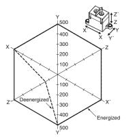
The value at which malfunction occurred was measured after applying shock to the test piece 3 times each in 6 directions along
