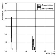
The switching performance and interruption performance were measured with a Zener diode and normal diode connected to absorb coil surge. These performances will be lower if only a normal diode is used.
