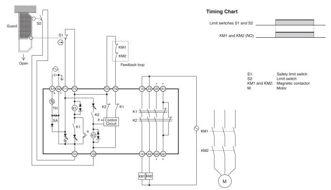
**Note:** External connections and timing charts for G9SB-200-B/301-B models are the same as those for G9SB-2002-A/3012-A models. \* Only the G9SB-3012-A model has terminals 33-34 and 41-42.
