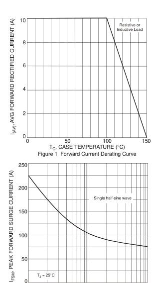
1 10 10 NUMBER OF CYCLES AT 60Hz Figure 3 Maximum Non-Repetitive Surge Current
