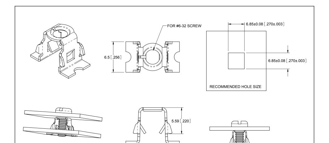
NOTES: 1. MATERIAL: 0.47 [.019] THICK SK-5 HEAT TREATED STEEL (RMS-338). FINISH: ZINC PLATED (RMS-337). ROCKWELL: "C" 40-45.
