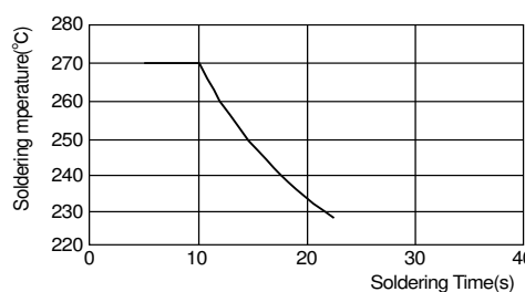
[Allowable Flow Soldering Temperature and Time]
