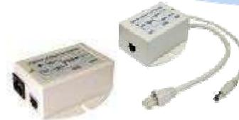
**Power Over Ethernet Injectors & Splitters**
