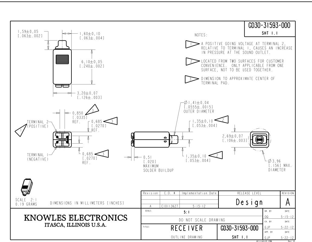
INTENDED FOR USE IN CIC, RIC, AND MINI-BTE APPLICATIONS. THIS IS A PAIR OF GE30 RECEIVERS WITH VERY LOW VIBRATION IN ALL DIRECTIONS. ONE GE30 RECEIVER IS REVERSE MAGNETIZED FOR MAGNETIC LEAKAGE CONSIDERATIONS. THIS RECEIVER HAS ANNEALED MUMETAL CUPS TO REDUCE MAGNETIC LEAKAGE.
