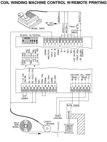
This application depicts a GEMINI 2000 controlling a coil winding machine. A length sensor provides output units in feet. Output 1 is used as the slow-down for the drive motor and Output 2 is used for the cut off knife control. A printer is used to record the length of each coil that is wound. Preset 1 is set to the slow down length and Preset 2 is set to the desired length of the coil.
