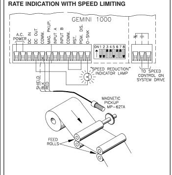
In this application, a GEMINI 1000 is used to indicate the speed of a printing press operation in feet/minute, while limiting the maximum speed to a desirable level.
