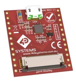
The gen4-PA incorporates the uUSB-PA5-II and gen4-IB together essentially, creating a single module with microUSB interface, and DIP style pads for GPIO breakout of all the signals used on the gen4 Display interface, which is useful for development or final product use. Standard 2.54mm (0.1") male pin headers can be mounted so the module signals can be interfaced to easily.
