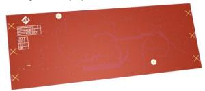
Where the Application PCB is shown to sit in Section 5.5, can house a small metal shield of the same size. This shield is used instead of, or underneath an Application PCB, to aid the on-board electronics in the prevention from potential RF or EMI signals.
