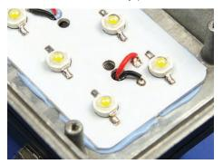
Gap Filler 3500LV is a two-part, high thermal conductivity, liquid gap filling material. This material offers the mechanical property benefits of a silicone material with the additional feature of low outgassing.
