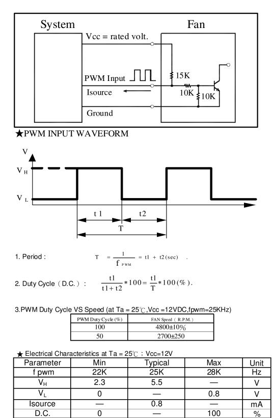
\* The speed is default to be maximum if PWM input pin is unconnected.
