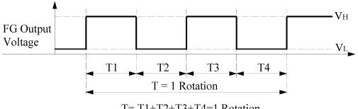
T=T1+T2+T3+T4=1 Rotation  $T=\frac{60}{\text{rpm}}$
