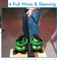
This completely modular system allows production level installation of braided sleeving over wire and cable bundles of virtually unlimited length. The system is simple to set up and interchangeable components accommodate diameters up to 2". For more information about this product contact your Account Representative.
