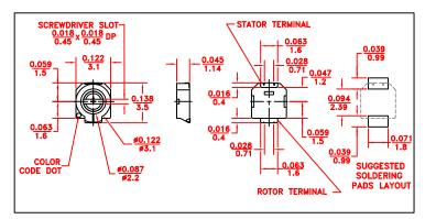
All dimensions are in/mm, unless otherwise specified, tolerance on dimensions  $\pm$  0.008/0.2
