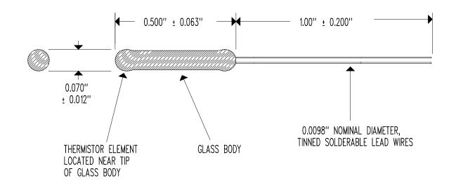
RESISTANCE @  $+25^{\circ}$ C = 2,000  $\Omega$  ± 5% RESISTANCE/TEMPERATURE CURVE = "F" BETA " $\beta$ " (+25 TO +85°C) = 3,499°K NOMINAL TEMPERATURE COEFFICIENT @  $+25^{\circ}$ C = -3.86%/°C NOMINAL TEMPERATURE RATING = -50 TO  $+300^{\circ}$ C
