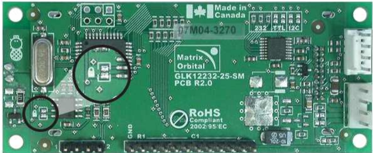
Figure 16: Filesystem Lock Jumper
