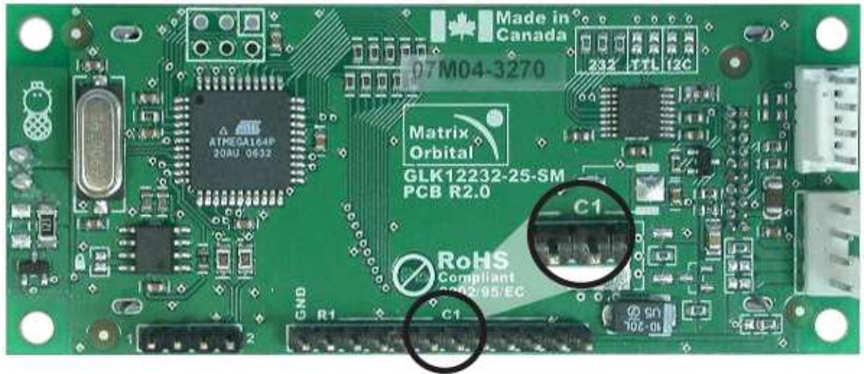
Figure 15: Manual Override Jumper
