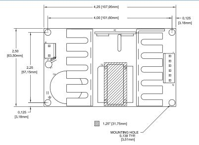
MAX. LEAD PROTRUSION 0.10" [2.54mm] MAX. COMPONENT HEIGHT 1.15" [29.21mm]
