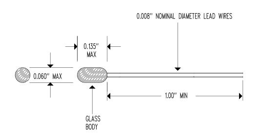
RESISTANCE @  $+25^{\circ}$ C = 10,000  $\Omega$  ± 1% RESISTANCE/TEMPERATURE CURVE = "G" BETA " $\beta$ " (+25 TO +85°C) = 3,695′K NOMINAL DISSIPATION CONSTANT = 0.75 mW/°C NOMINAL (STILL AIR) THERMAL TIME CONSTANT = 0.35 SECONDS NOMINAL (STIRRED OIL) MAXIMUM TEMPERATURE RATING =  $+250^{\circ}$ C
