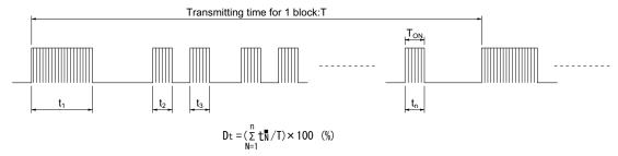
In case the signal format of total duty and/or ON/OFF signal time dosen't meet the conditions noted above, there is a case that reception distance much reduces or output dose not appear.
