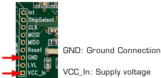
Figure 2.5 External power supply via J19
