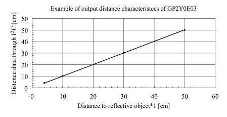
Example of output distance characteristics of GP2Y0E03
