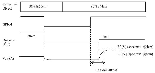
Response time of I<sup>2</sup>C output is faster than that of Vout(A) because it is stabilized soon after distance data output. Distance data is updated every 2ms after response time.
