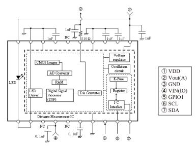
Please use an electric source with an output current of 150mA or more because LED pulse current is more than 100mA.
