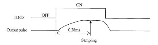
3-4 Recommended input condition for LED input terminal
