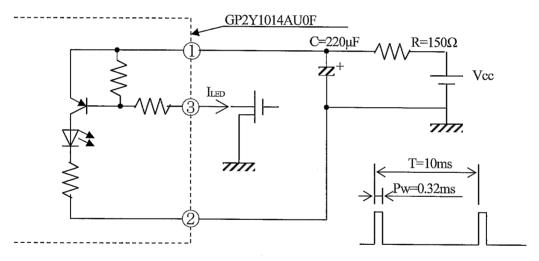
(\*4) Sampling timing of output pulse
