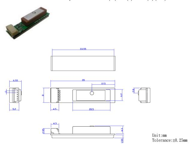
The dimension of GP-735 with I-PEX connector is  $8(W) \times 35(L) \times 5.2(H)$  (mm).
