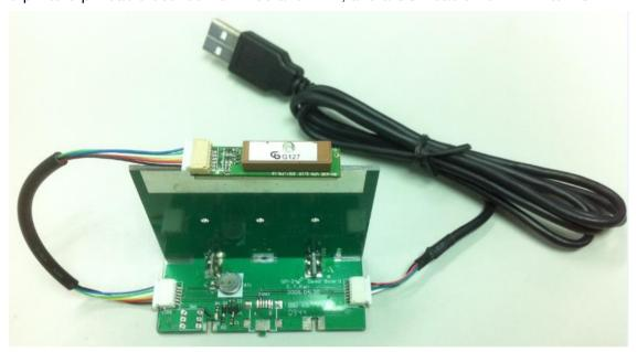
Large ground plane below GP-735 boots its performance. As shown in following picture, GP-735 mounts on top of EVB and the shielding case of GP-735 is soldered to the ground plane of EVB. GP-735 should face up to the sky.
