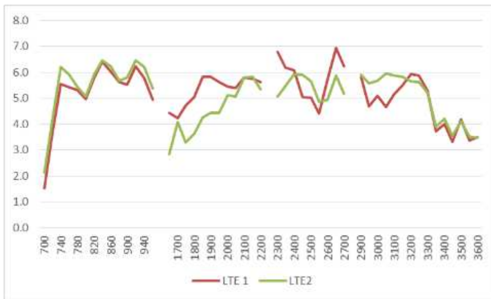
Maximum 3D gain, LTE antenna with 2ft metal plate and 4inch cables
