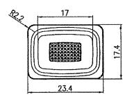
LED 12VDC 14V w/resistor R=680 ohm
