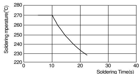
[Allowable Flow Soldering Temperature and Time]
