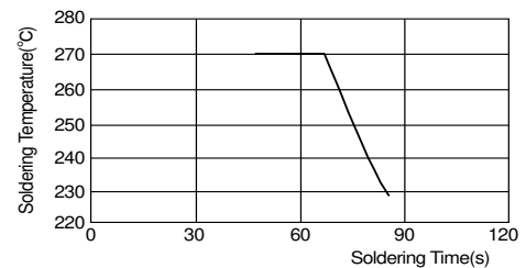
[Allowable Reflow Soldering Temperature and Time]
