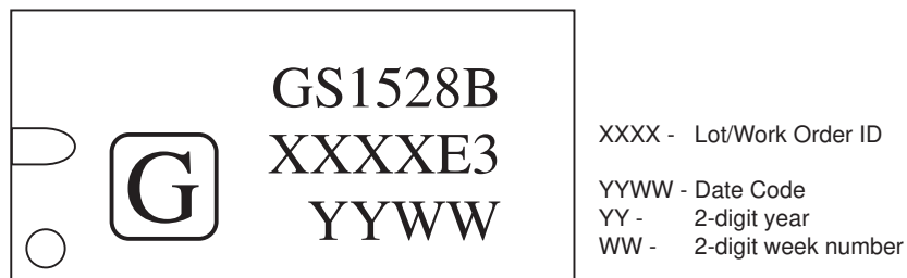
Figure 7-2: GS1528B Marking Diagram
