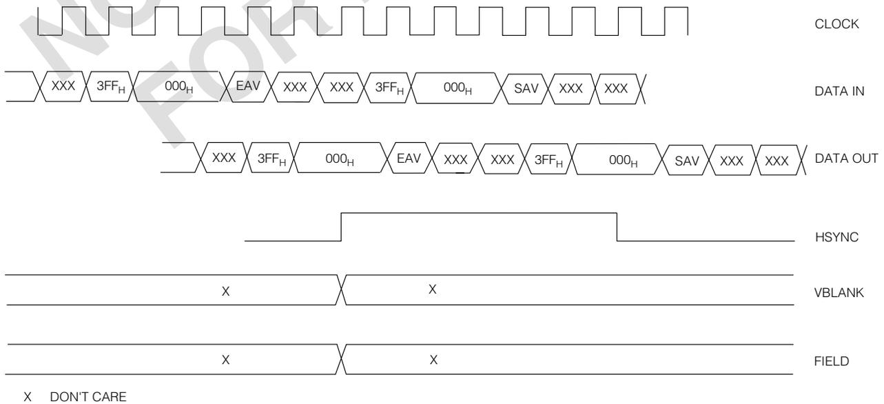
Fig. 5 Component Timing Signals
