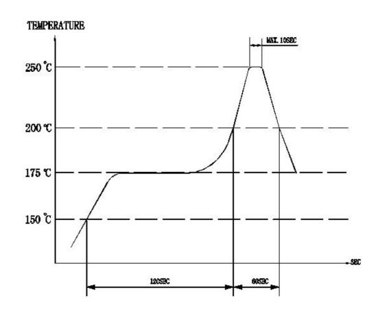
Heat resistant line (Use when heat resistant reliability test is performed)
