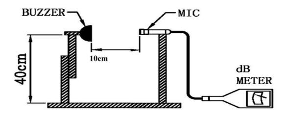
MIC: RION S.P.L meter UC30 or equivalent S.G: Hewlett Packard 33120A Function Generator or equivalent
