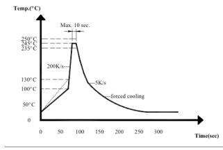
Recommendable wave soldering condition is as follows:
