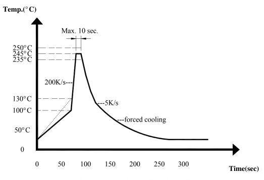
Recommendable wave soldering condition is as follows.
