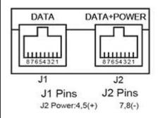
PoE injector wiring Data, Data+Power, RJ45 x 2
