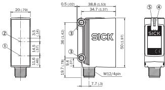
① Center of optical axis, sender
