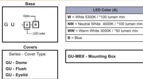
\* LED flux data is manufacturers test data @ 25°C T<sub>J</sub>. Light output at max acceptable ambient temp will be approximately 25-30% lower, depending on thermal conductivity of mounting surface and lens type.
