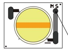
Please take note of the following, when measuring case temperature. 1 The LED device mounting surface should be flat/plain surface. 2 The substrate surface temperature should be uniform.
