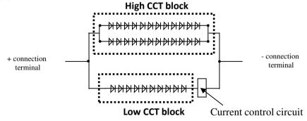
High CCT block 12 series  $\times$  2 parallel = 24 pcs of LEDs
