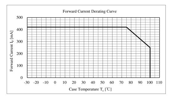
(Note) To keep the case temperature lower than the rating, enough heat-radiation performance needs to be secured by using an adequate heat sink.
