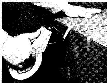
Figure 4 — Pull the H-131 over the box edge to dispense about 2 inches [50 mm] of tape as shown. Apply tension on the brake, tilt the H-131 upward, and tack the tape to the side of the box with the top buff pad to form a tight seal.
